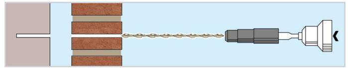
2. Load tie into DryFix Power Driver Attachment fitted to SDS hammer drill
